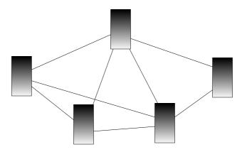
The figure above shows how systems connect to each other in a point to point architecture and that the number of connections could be as high as  $(n^{2-} n)/2$ , although in reality, not all the systems need to connect to each other. In a typical enterprise organisation with tens or perhaps hundreds of systems requiring integration, the number of interfaces that are required soon becomes unmanageable.
