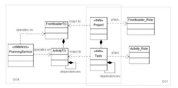
Figure 1: Class Diagram showing classes involved in both the DCI and SOA solutions to the frontloader example.
